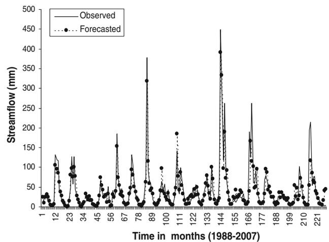
**Fig. 4** Comparison of observed data with predicted data using the ARIMA model
