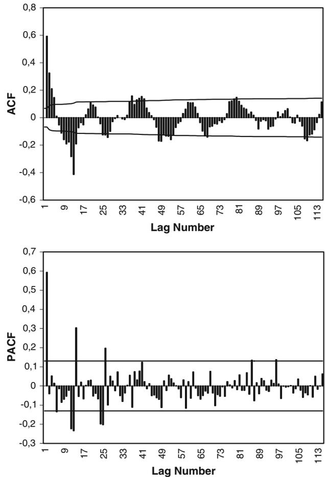
**Fig. 3** Autocorrelation function (ACF) and partial autocorrelation function (PACF) plots of seasonal differenced time series
