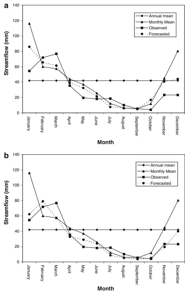
**Fig. 5** Comparison of observed and forecasted streamflow from model 1 (a) and 3 (b) and two drought truncation levels
